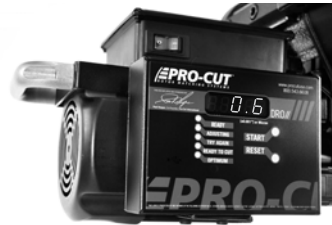
| This display of final compensation equals .0006"
