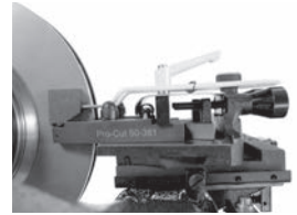
The chip deflector reduces vibration and must be used on EVERY cut.
